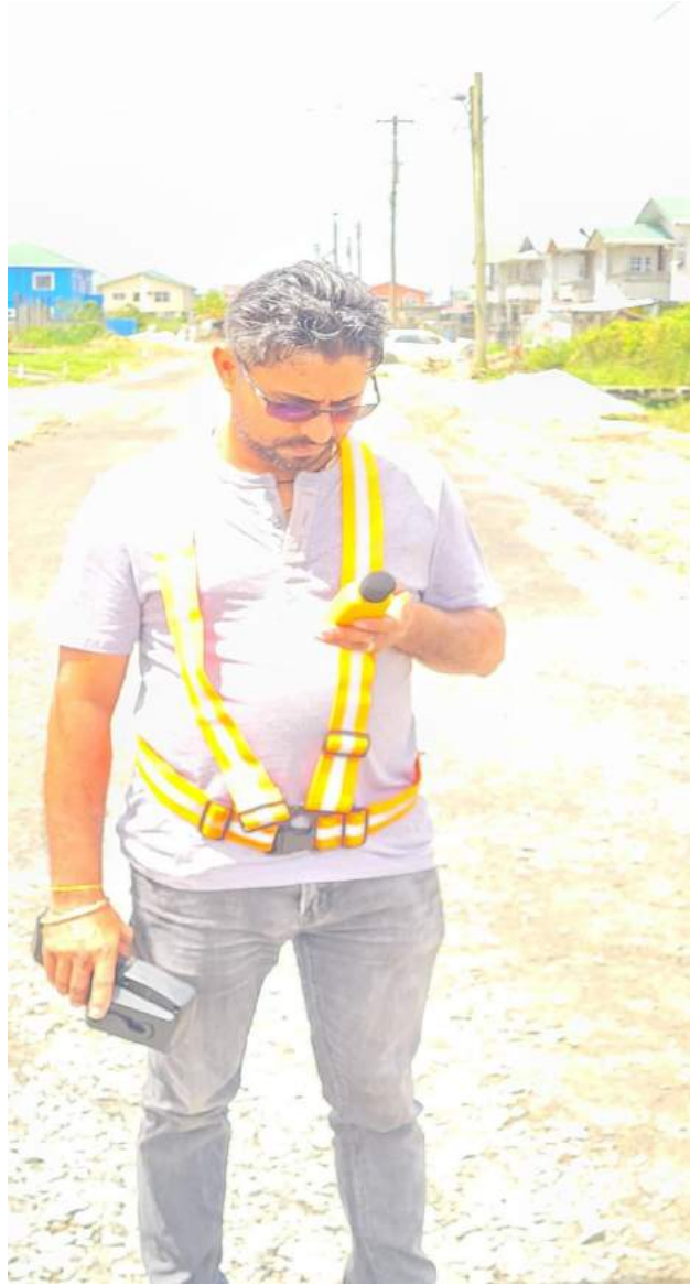
Figure 4-5: Conducting Noise Measurement within the Project Area
